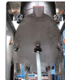
Quick release toggle clamps to access product chamber for cleaning and maintenance.
