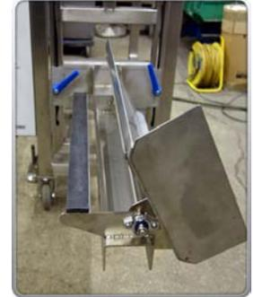
Adjustable height tilting sack support to reduce manual handling.
