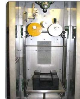
Internal mechanical weighing mechanism of the S1000GR.
