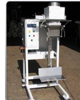
Fitted with an interchangeable open mouth bag filling attachment.
