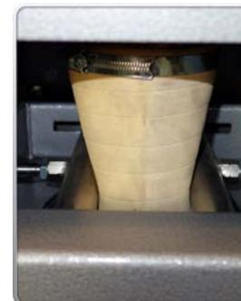
Pneumatic pinch valve assembly to control product feed flow rate.
