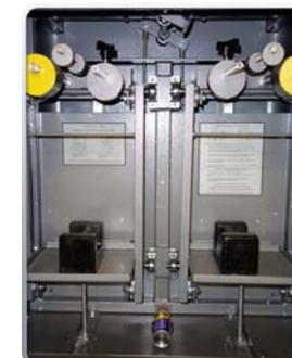
Internal mechanical weighing mechanism of the S2000GR.
